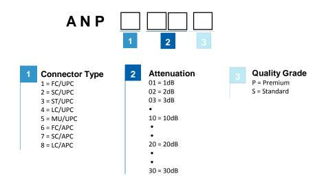
*Example:* Ordering code : ANP-2-05-S Item Description: Plug Type Attenuator SC/UPC 5dB, Standard Grade
